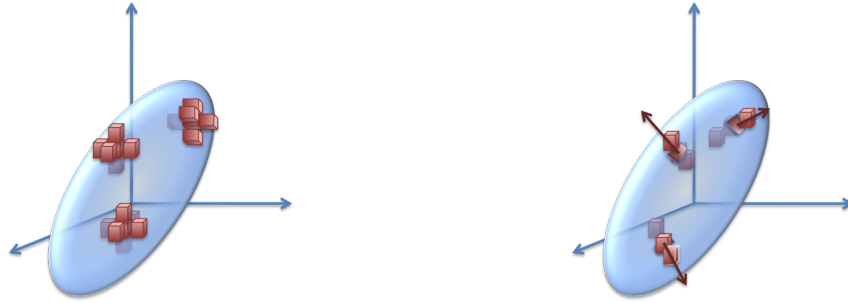
Figure 3.3: A neighborhood system comparison between a traditional (left) and an adapted (right) system: A traditional neighboring system considers 8 directions regardless of structures position while the adapted system here considers only two along the gradient descents direction of structure priors.
